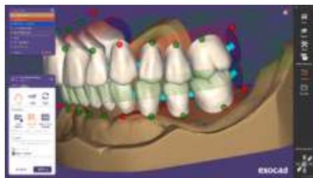
Fig . 4: Customization of prosthetic posterior teeth: Greater flexibility is provided because posterior teeth can now also be individually adjusted in the set-up of full dentures.
